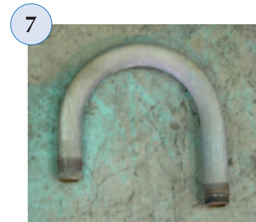
Center pivot gooseneck elbow for new drop tubes
