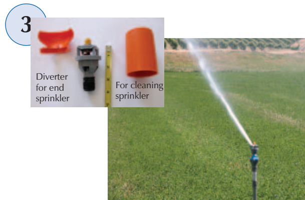
Low pressure rotating sprinkler to replace impact sprinkler (example shown of ‘wind fighter’ sprinkler by Nelson)
