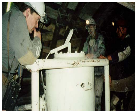
Ukraine Mine Safety: After installation of equipment, the percentage of non-combustible material found in the exposed areas that had been rock dusted increased by 84.8%.
