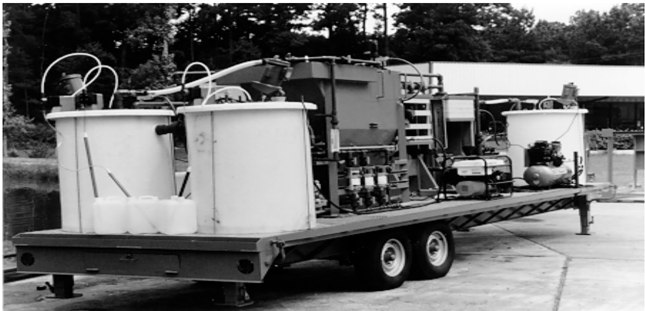
Mobile CPFM® Unit, Including Mixing Tanks, Pumps, Filter Apparatus, and Other Equipment
