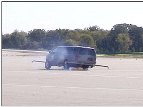
Figure 6.1. One of three “spin-outs” observed during 2003 Ford E-350 Slowly Increasing Steer tests performed with left steering, Placard tire inflation pressures (55-psi front / 80-psi rear), and Maximum Occupancy loading.
