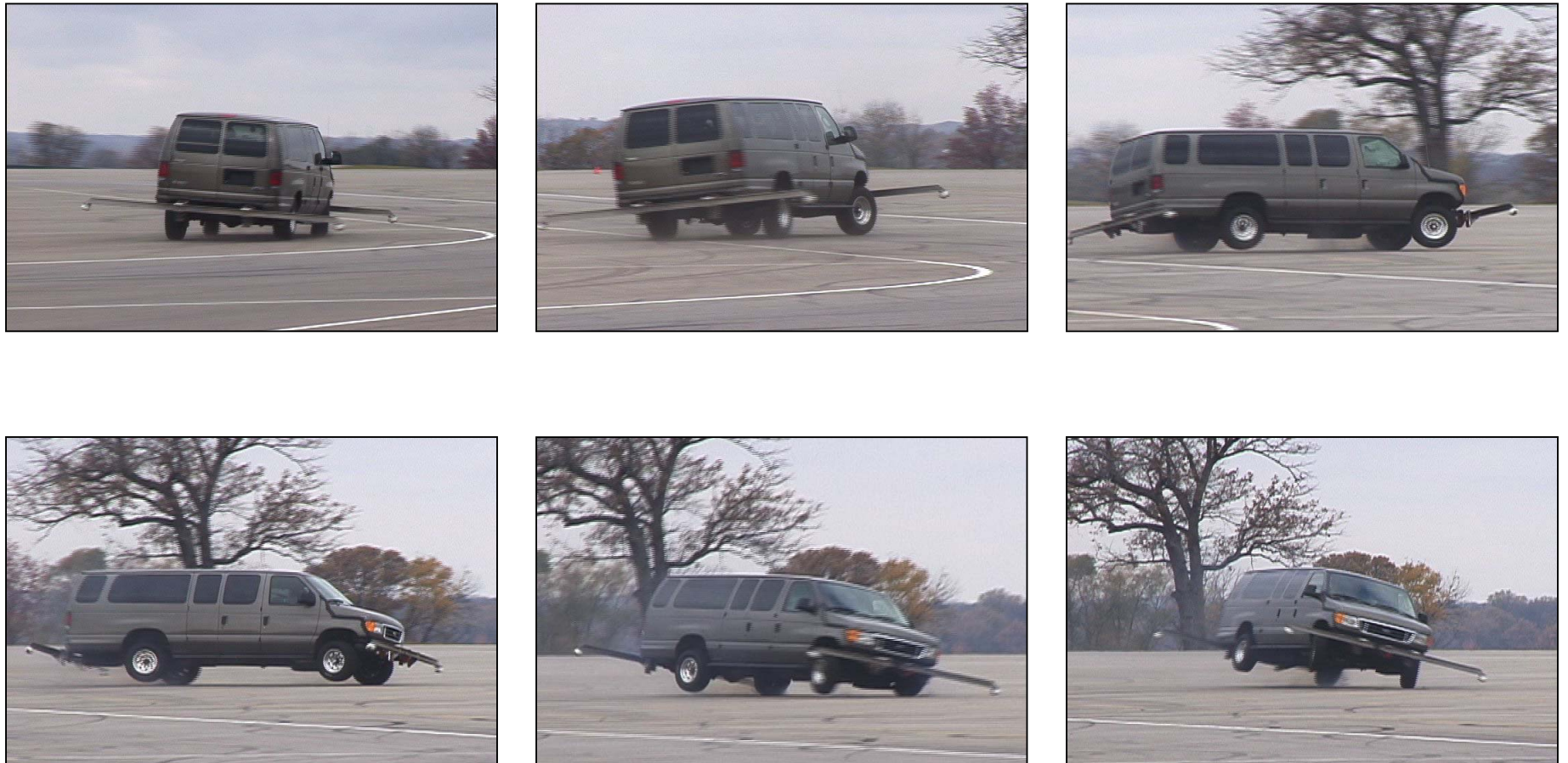
Figure 7.1. Two-wheel lift produced during a 5-occupant, left-right Road Edge Recovery maneuver initiated at 49.5 mph with a 2003 Ford E-350. Tires were inflated to the Current MAP pressures (46-psi front, 60-psi rear).
