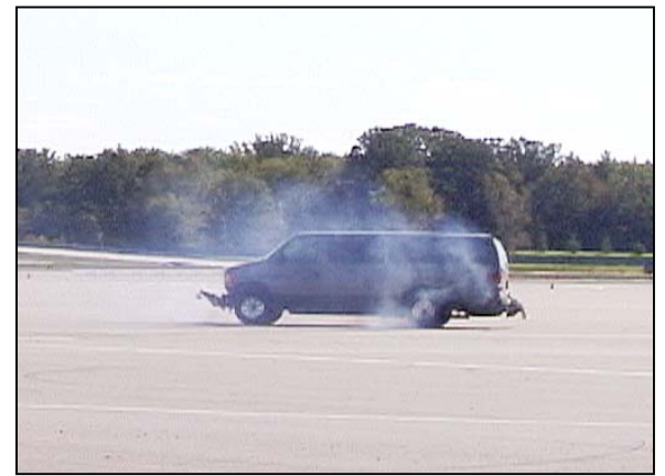
Figure 6.1. One of three “spin-outs” observed during 2003 Ford E-350 Slowly Increasing Steer tests performed with left steering, Placard tire inflation pressures (55-psi front / 80-psi rear), and Maximum Occupancy loading.
