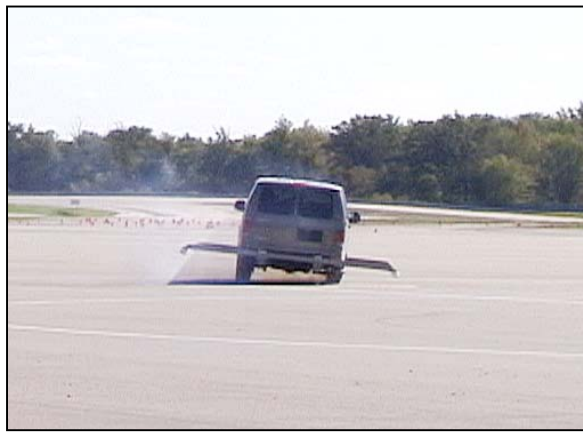
Figure 6.1. One of three “spin-outs” observed during 2003 Ford E-350 Slowly Increasing Steer tests performed with left steering, Placard tire inflation pressures (55-psi front / 80-psi rear), and Maximum Occupancy loading.
