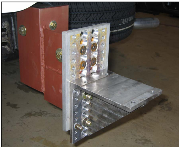
Figure 3.2. “Heavy-Duty” outrigger bracket installed at the left rear of a 2004 GMC Savana 3500.
