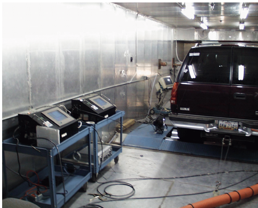
Figure 3-1. Chevy Tahoe in Dynamometer Cell
