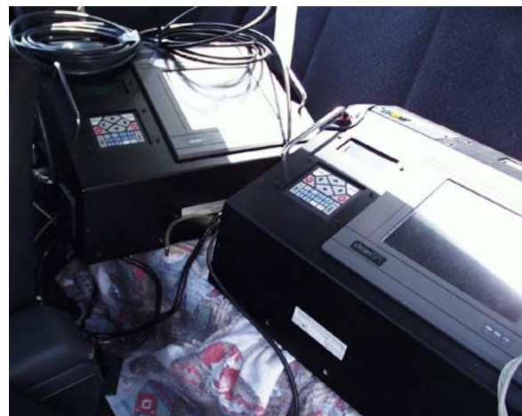
Figure 3-3. View of the Duplicate REMOTE OEMs in the Chevy Tahoe Before On-Road Testing
