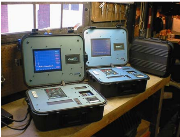
Figure 2-1. Clean Air Technologies REMOTE On-Board Emissions Monitor
