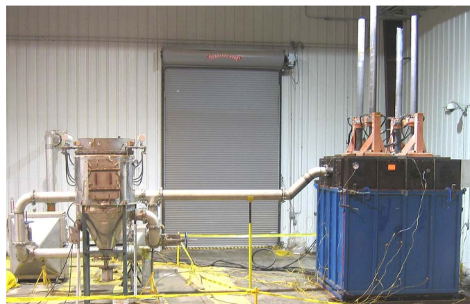
GeoMelt™ ICV process. Source: Ref. 24
