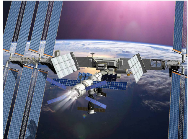
Artist's impression of the ATV reboosting the ISS to a higher orbit
