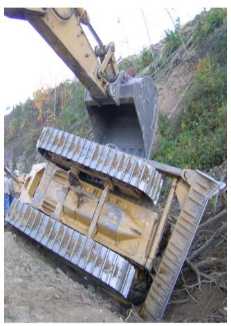
On October 22, 2008, a dozer operator was fatally injured when the dozer he was operating slipped and rolled sideways down a steep 80 foot incline coming to rest on its left side. This was the fourth accident in five weeks where a dozer operator was either fatally injured or suffered serious life threatening injuries. (See Picture to the Left)
