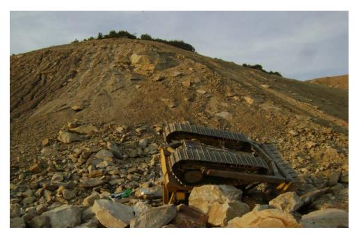
On September 19, 2008, a dozer operator was killed when the dozer he was operating flipped over and rolled approximately 180 feet down a slope. (See the Picture Above)
