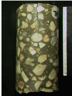
Figure 1. Core from bridge deck showing vertical surface cracks induced by general expansion and cracking in the interior.
