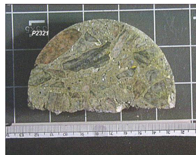
Figure 5. Lapped section from core of damaged bridge deck treated with sodium cobaltnitrite.
