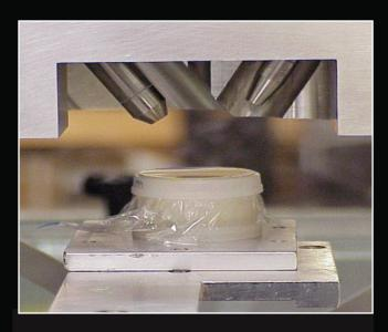
The Confocal X-Ray Fluorescence Microscope, a 2004 R&D 100 Award winner, can measure elemental concentrations, e.g., number of layers of paint, composition of each layer, and the order of application as a function of depth at any point on a fine-art painting, helping historians determine condition and authenticity of a painting.
