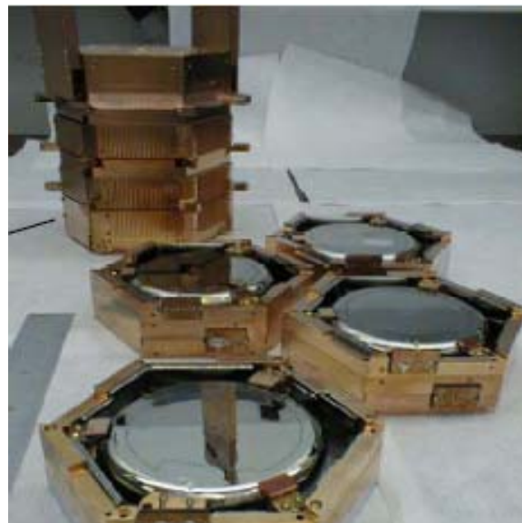
Four of the Silicon and Germanium detectors in their mounts at the Soudan mine in Minnesota. Credit: University of California, Berkeley.
