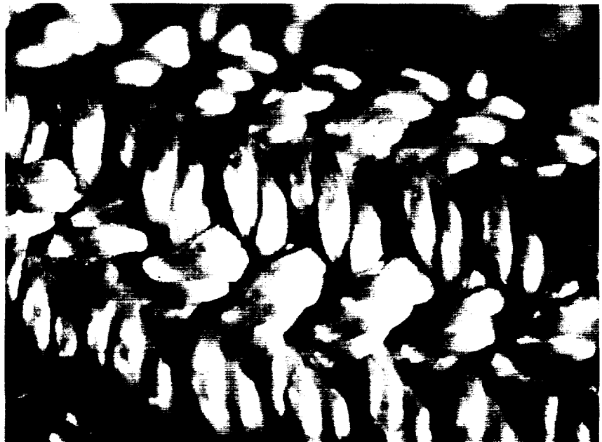
FIGURE 2.—Enlarged view (magnified 20 \times ) of woven glass fabric; black particles are believed to be Moon dust.
