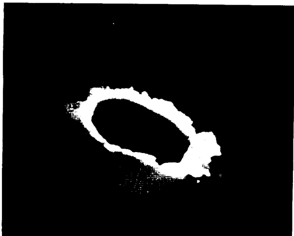
FIGURE 5.—A 3- \mu m-wide crater in control sample. The crater was formed by iron particles at a velocity of 3 to 6 km/sec.
