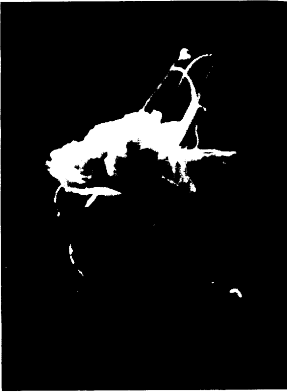
FIGURE 2.—Scanning electron microscope photograph of the particle in figure 1. Note the structural change in the whiskers caused by the vacuum deposition processes.
