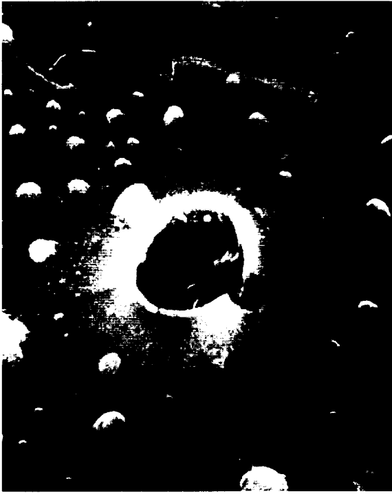
FIGURE 2.—SEM photograph of 3- \mu\text{m} crater produced in glass by a 6-km/sec carbonyl iron sphere.
