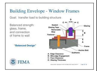
To retain the glass in the frame, a minimum of a ¼-inch bead of structural sealant (i.e., silicone or polyvinyl butyral) should be used around the inner perimeter of the window. This should be done on all four sides of the window. Since strip windows with butt glazing can only apply sealant on the top and bottom, they are not good options for blast as the bite must be large, even with sealant.
