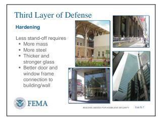
U.S. Embassy: Kampala, Uganda designed to resist explosive blast [upper left – DOS and Hinman]. Other three photos are from New York City indicating glass and overhang (poor) [lower left], similar glass and overhang (poor) but with wall (better) [upper right], and window curtain wall (usually poor) [lower right]. VISUAL X-8
