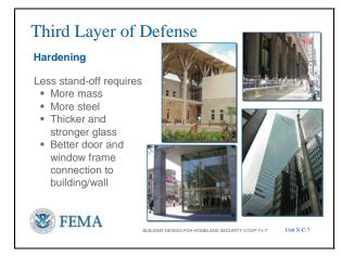
U.S. Embassy: Kampala, Uganda designed to resist explosive blast [upper left – DOS and Hinman]. Other three photos are from New York City indicating glass and overhang (poor) [lower left], similar glass and overhang (poor) but with wall (better) [upper right], and window curtain wall (usually poor) [lower right]. VISUAL X-C-8
