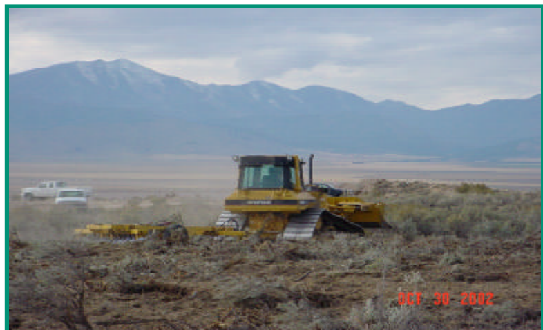
The type of equipment used to disc sagebrush on West Mountain. Followed by seeding, this treatment will allow fire resistant and native plants to grow in areas were sagebrush and non-native grasses have encroached.
