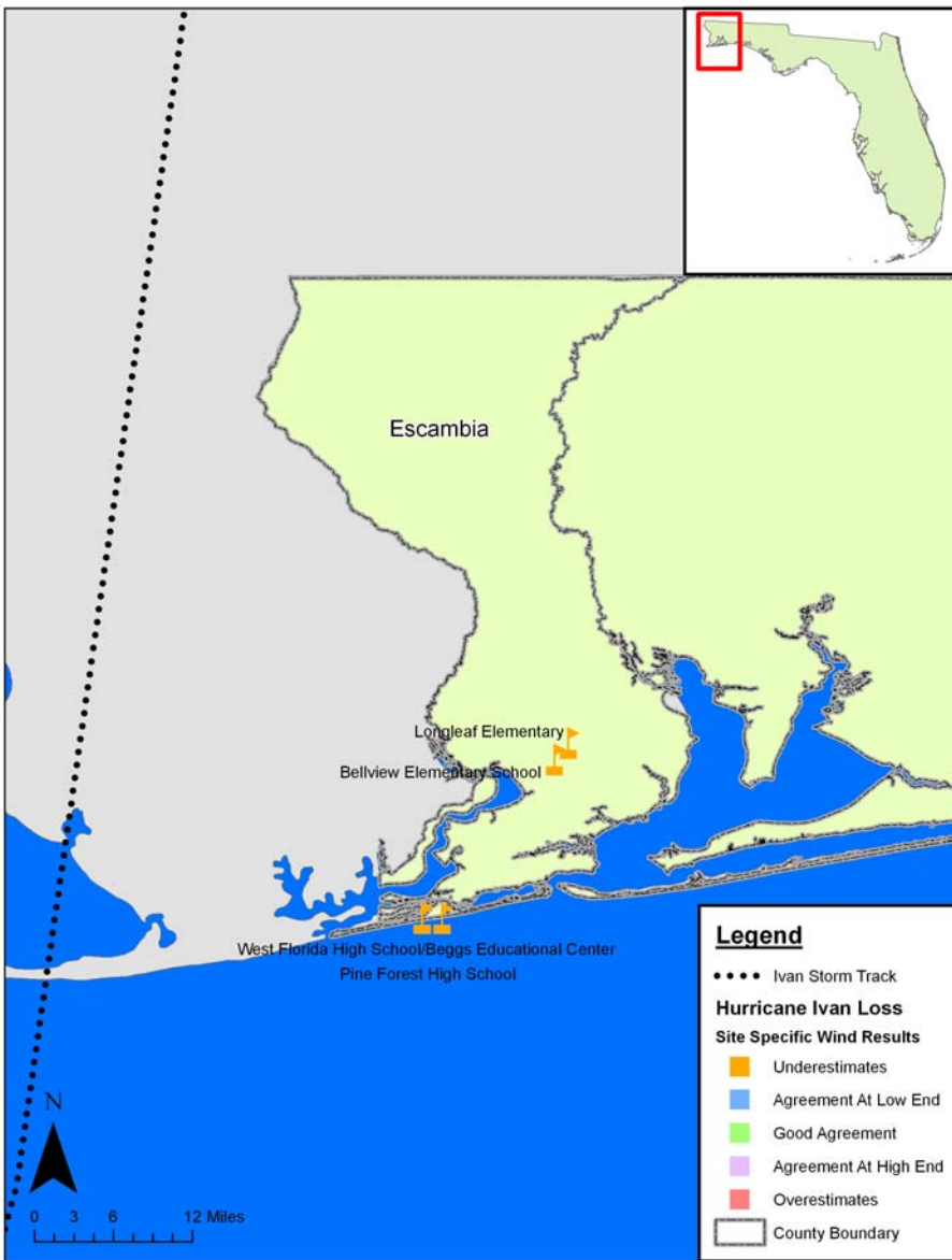
Figure 17. Hurricane Ivan Economic Loss - Comparison of Observed Site Specific Critical Facility Loss and HAZUS-MH Wind Loss Curve
