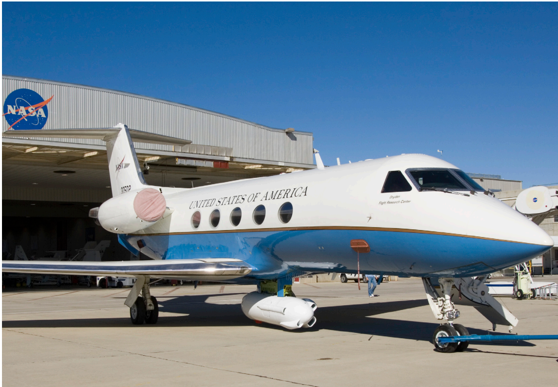
NASA Dryden's Gulfstream-III with the UAVSAR underbelly pod.
