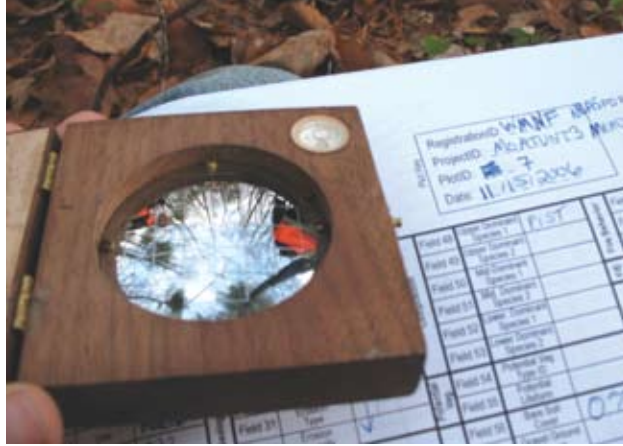
Canopy mirror used to measure openings in the forest canopy. WMNF photo by Erin Small.
