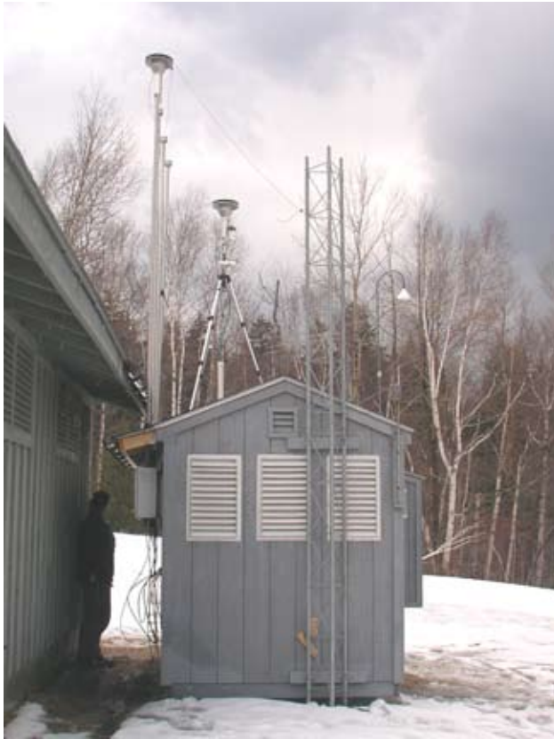
The IMPROVE site at Camp Dodge monitors air quality on the Forest. (WMNF photo by Livia Crowley)
