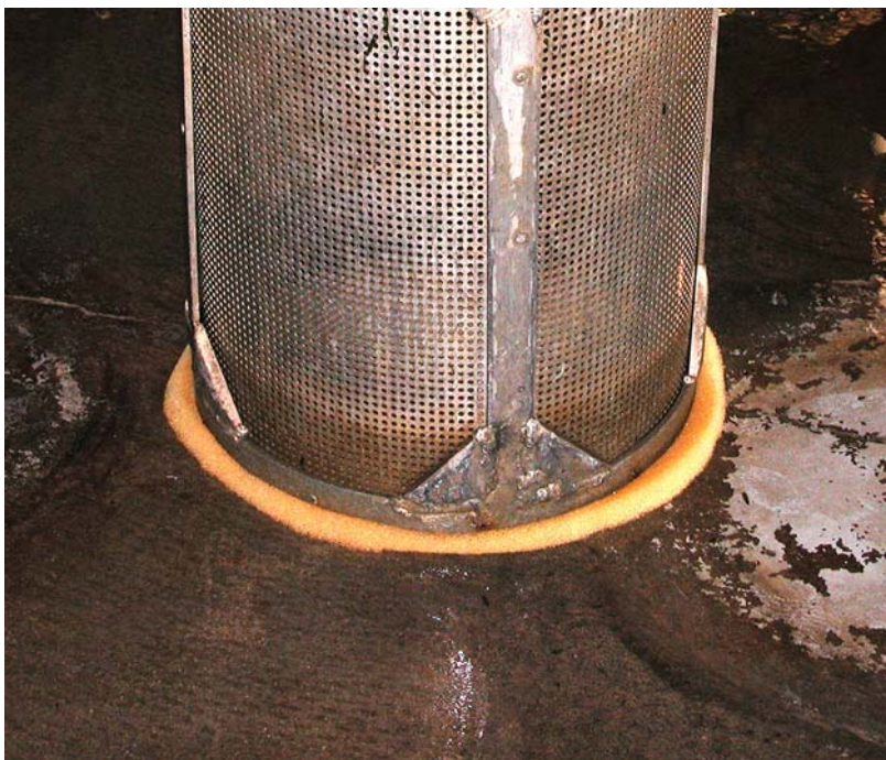
FIGURE 5.—Foam pad used to seal the bottom rim of the 10-minute-count screens.
