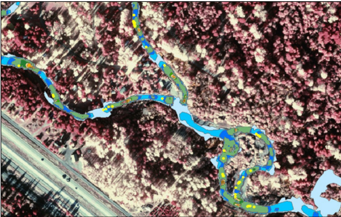
Figure 11: Aerial photograph of the Easton reach showing the Froude number classification and redd locations (yellow dots). Flow direction is west to east. The legend from Figure 9 applies. (Figure courtesy of Ken Bovee.)
