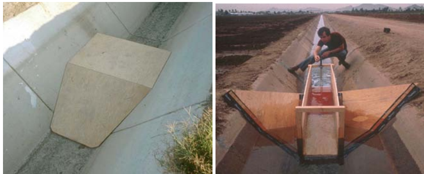
Figure 9. — Temporary Flumes for Lined Trapezoidal Channels.
