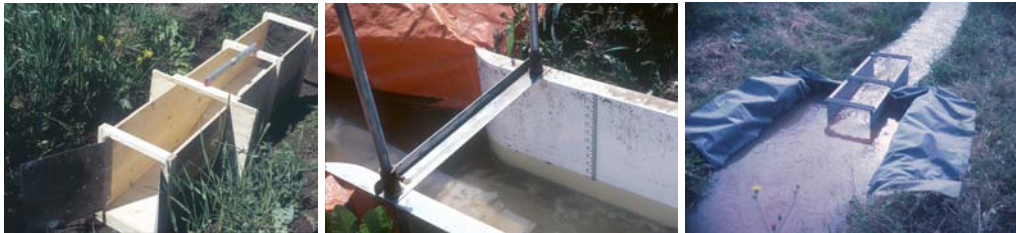
Figure 8. — Rectangular-Throated Portable Flumes.
