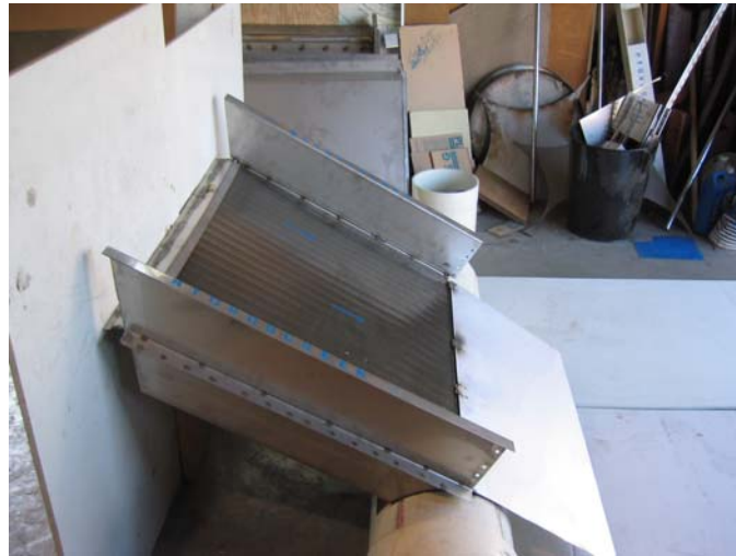
Figure 13. — Coanda-effect screen structure in the shop, configured to discharge directly into a PVC pipe.
