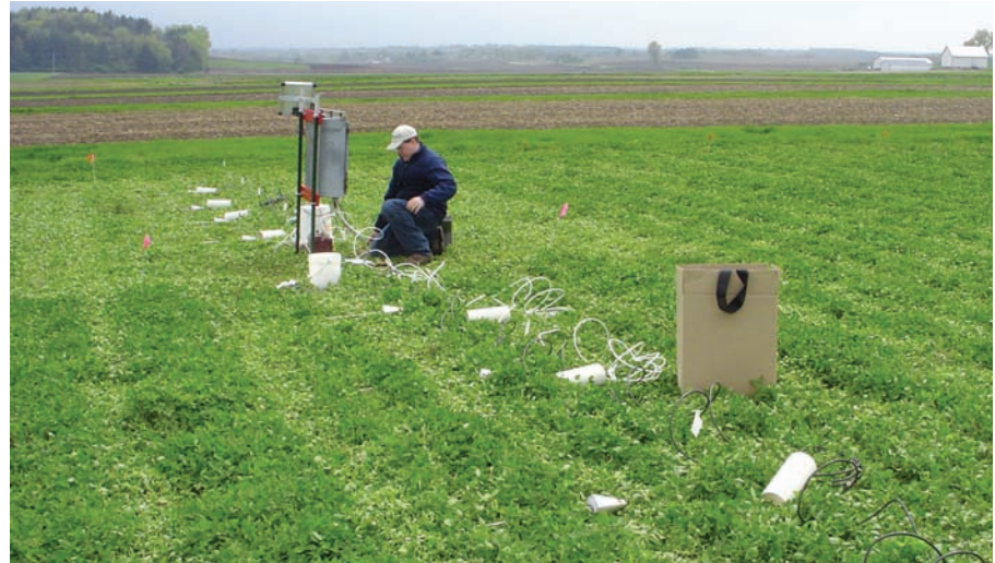
ARS technician Todd Schumacher installs soil moisture monitoring equipment in a kura clover living mulch experiment at a University of Wisconsin research farm in Arlington, Wisconsin. Row locations of recently planted no-till corn are evident from the effects of band-applied herbicide directly over the rows.
