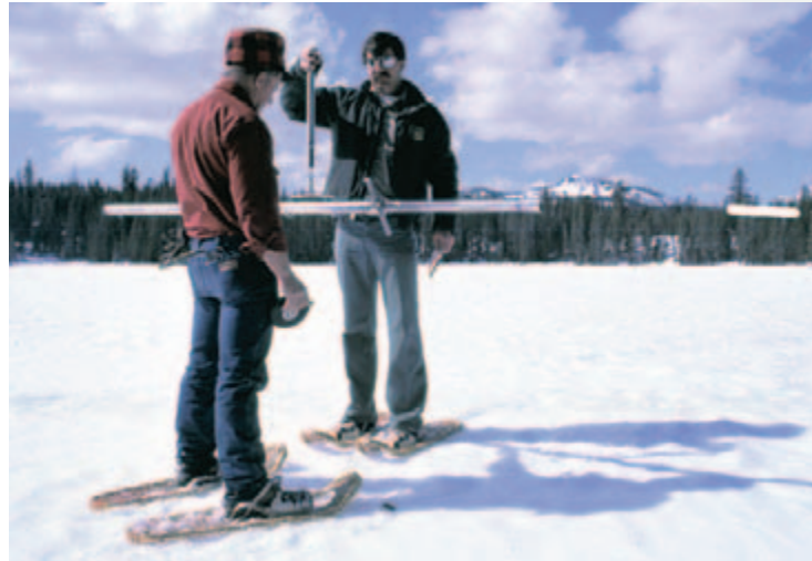
Measuring snow for water content at Silver Lake on the Almanor Ranger District
