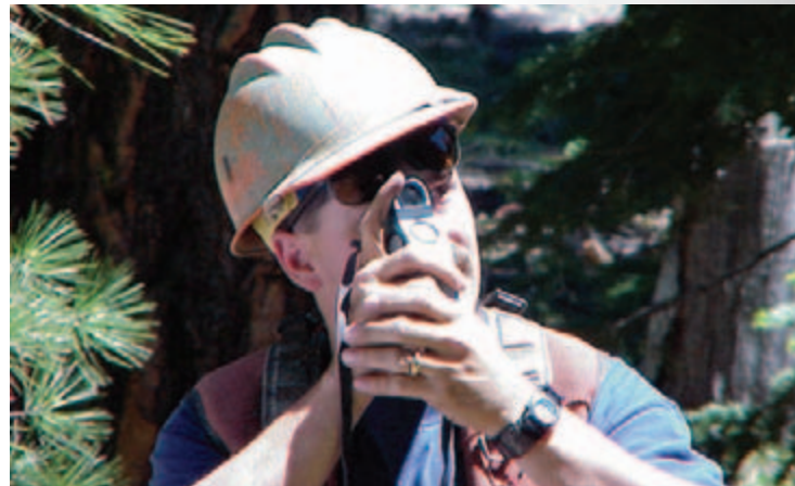
Measuring tree height with a relaskop
