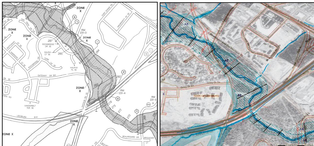
Figure 1. In these sample flood map panels, the enhanced detail shown on the digital map (right) can be compared to the older paper map (left).
