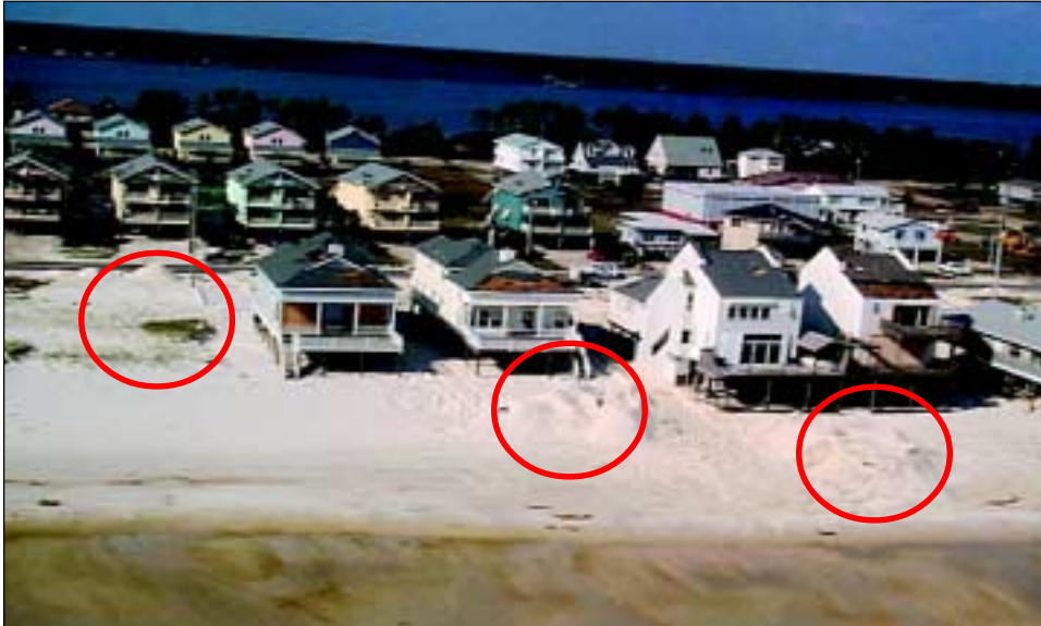
FIGURE 5-6 Excess sand (circled) from beneath houses and on roadways that was returned to the beach.
