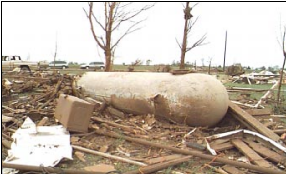
FIGURE 3-20: Wind displaced this very large propane tank in Bridge Creek, Oklahoma; its original location could not be determined. This area was hit by the vortex of a violent tornado.
