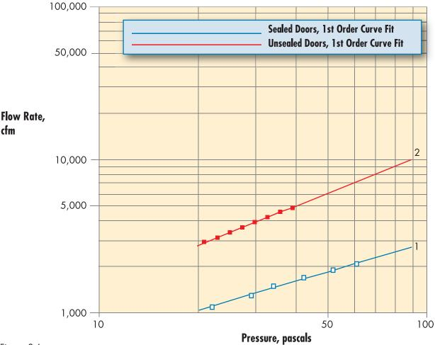
Figure 3-6 Blower-door test results on the stairwell selected for a safe room SOURCE: BATTELLE
