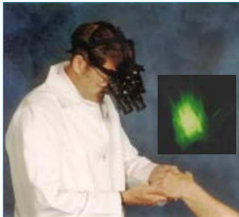
Using night vision goggles and AFRL's vein viewing device, a researcher sees beneath the skin to inspect the vasculature of a hand.
