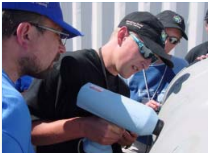
The Acoustic Inspection Device allows inspectors to quickly and easily determine the contents of a container. This noninvasive method of examining sealed containers and verifying contents is significantly safer and faster than conventional inspection methods.
