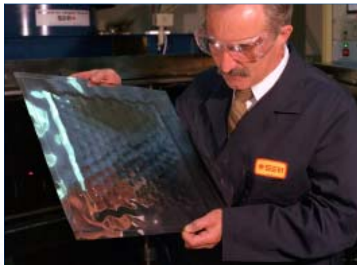
Compact vacuum insulation (CVI) is one of the important technologies incorporated into the catalytic converter. CVI is not only essential to minimizing cold-start emissions, it also has many other applications that range from refrigeration to cooking utensils.
