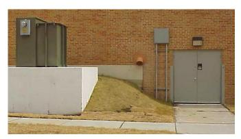
In addition to elevating electrical equipment (left), engineers also outfitted 24 major doors and windows (right) with special metal shields that can be attached ahead of time to keep out floodwaters.
