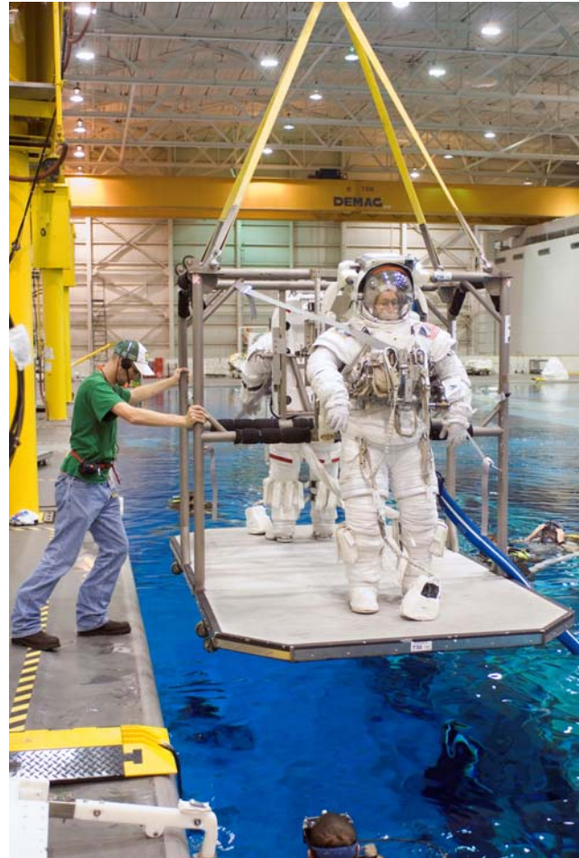
Astronauts Sandra H. Magnus, Expedition 18 flight engineer, and E. Michael Fincke (partially obscured), commander, are about to be submerged in the waters of the Neutral Buoyancy Laboratory (NBL) near NASA's Johnson Space Center. Magnus and Fincke are attired in training versions of their Extravehicular Mobility Unit (EMU) spacesuits.
