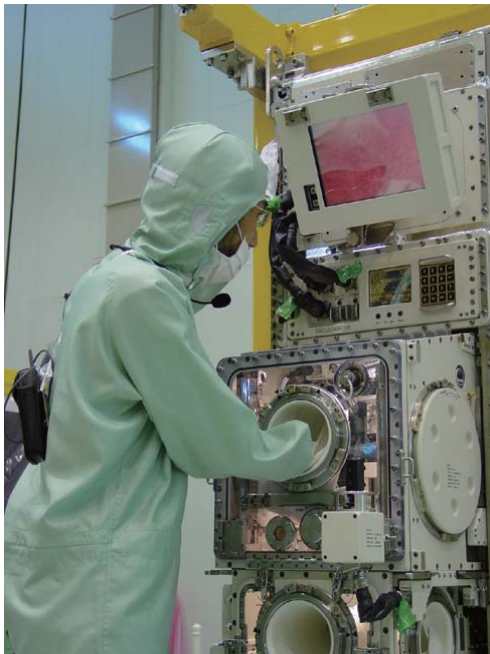
Clean Bench (CB) in SAIBO rack
