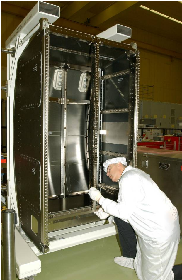
International standard payload rack into which experiment facilities, subsystems or storage racks can be fitted.
