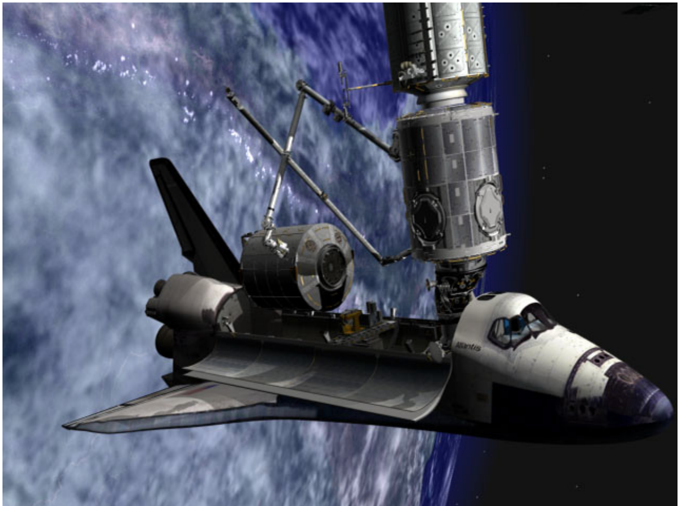
This image illustrates the Columbus laboratory being grappled by the Station Robotic Arm, Canadarm2, in preparation for its relocation to its permanent location.
