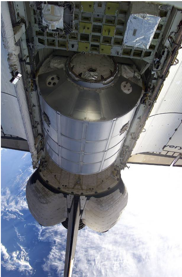
Multi-purpose logistics module 'Leonardo' in the space shuttle cargo bay on March 10, 2001, during the STS-102 mission to the ISS.
