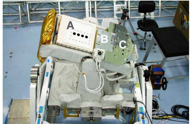
The SOLAR facility with the three different instruments highlighted. A is SOLSPEC, B is SOL-ACES and C is SOVIM.
