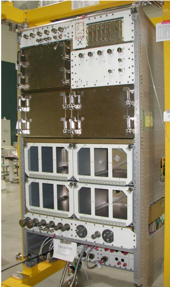
European Drawer Rack with clear view of 3 drawer and 4 locker locations
