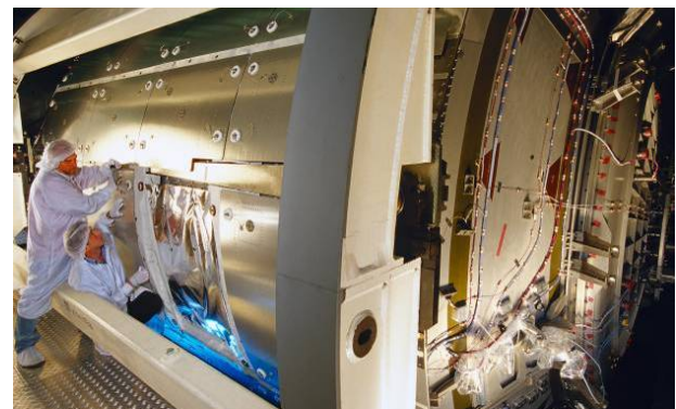
Columbus Laboratory at EADS Astrium in Bremen with debris protection panels. Insulation material exposed under one section of paneling. July 2004.
