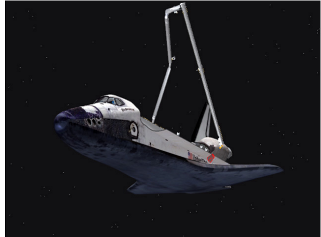
This graphic illustrates the inspection Endeavour's astronauts will perform using the Orbiter Boom Sensor System.
