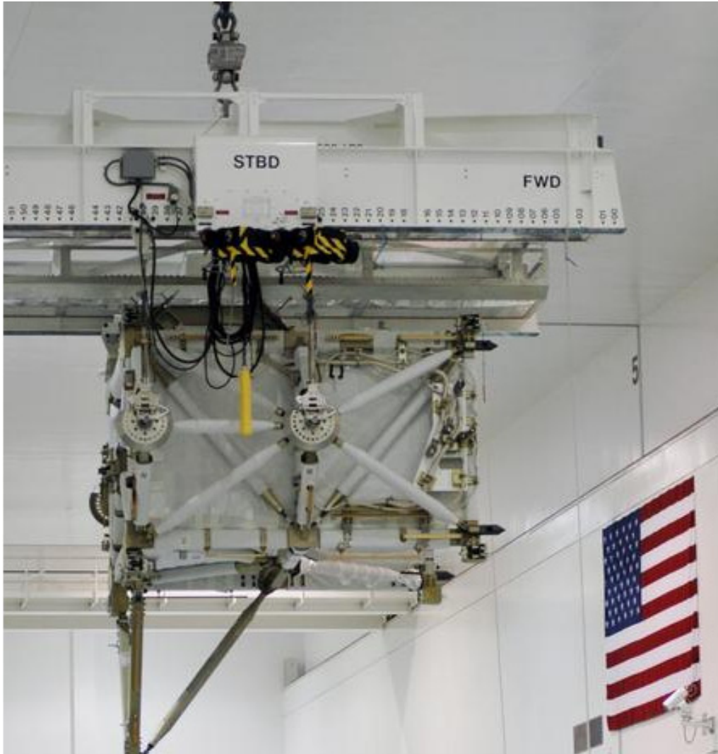
The S5 short spacer is shown in the Space Station Processing Facility at Kennedy Space Center.
