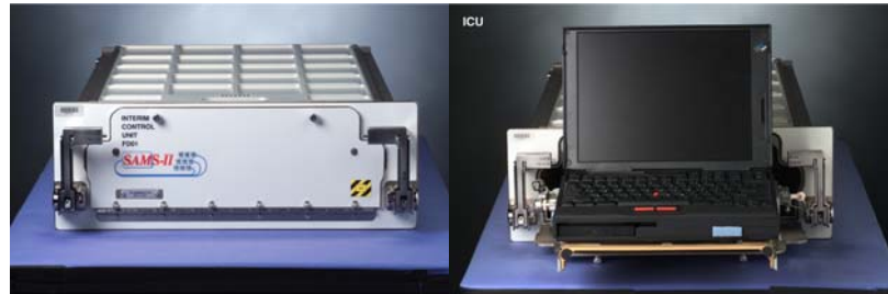
SAMS Interim Control Unit to left, SAMS ICU with laptop on right
