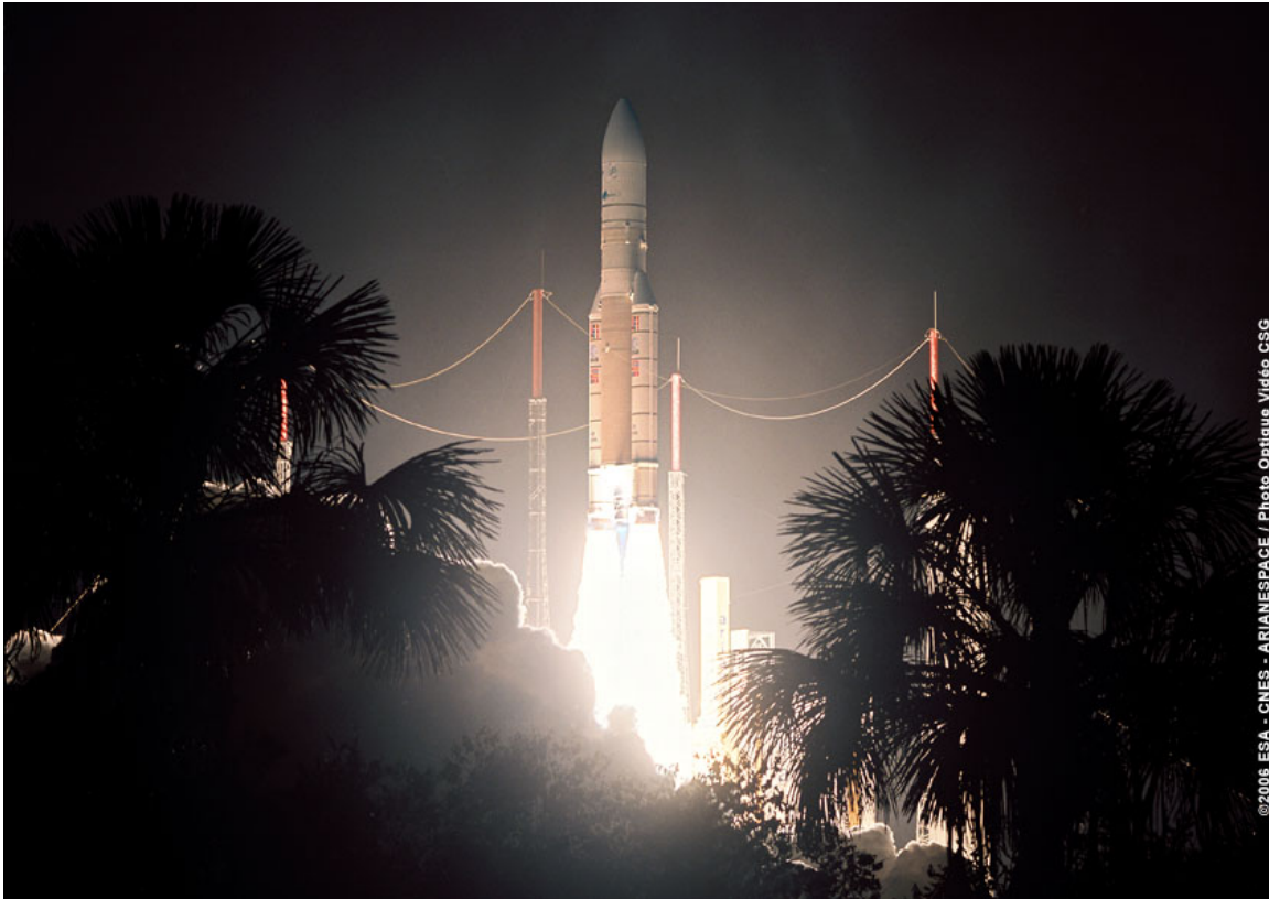
An Ariane 5 rocket clears the launch tower as it climbs out under the power of its Vulcain main engine and its two solid rocket motors.
