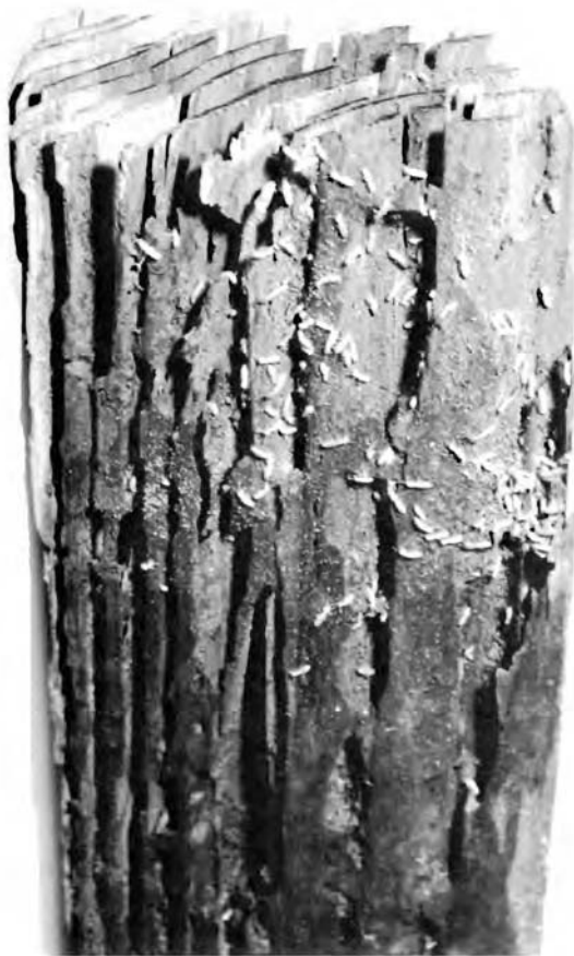
Figure 3.—Pine 2x4 destroyed by termites.
