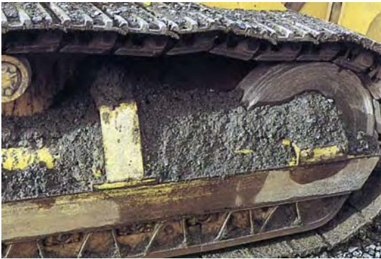
Figure 5 – Muddy tractor wheel and track assembly that may transport P. lateralis from an infested site.
