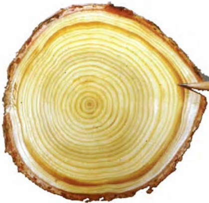
Fig. 5: Compression-like wood in irregular outer rings caused by the trees reaction to feeding by the balsam woolly adelgid.
