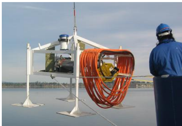
Figure 2-11 Representative Junction Box (Jbox)
