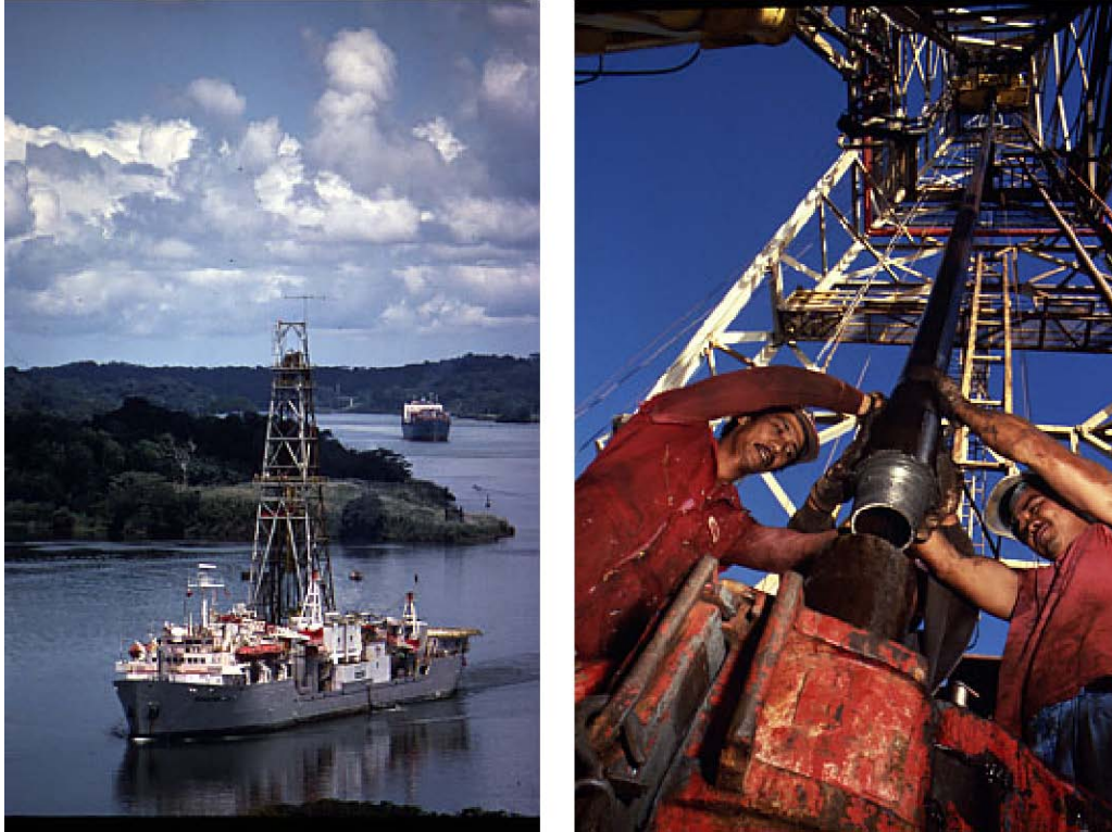
(Left) JOIDES Resolution (originally known as SEDCO/BP 471) was converted in Pascagoula, Mississippi, in the fall of 1984. She was built in Halifax, Nova Scotia in 1978 and had previously sailed the world as a top-class oil-exploration vessel. (Right) The ship can deploy up to 30,000 feet of drill string.
