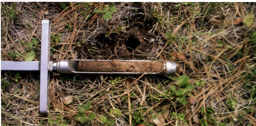
A soil sample collected from a forest is shown. The darker color at the surface is due to soil organic carbon.
