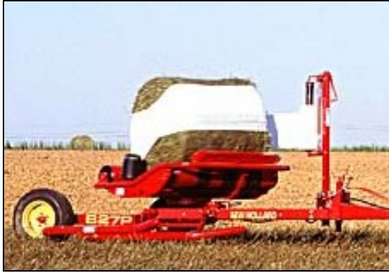
Figure 9-3. Bale wrappers tightly seal each bale of hay in plastic for storage. (Courtesy of New Holland.)
