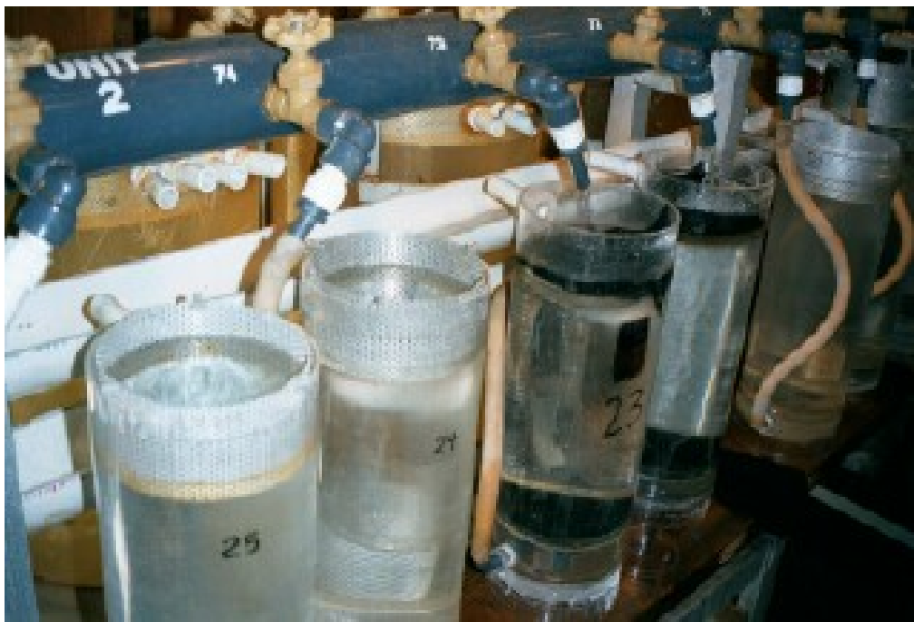
Photo 3. McDonald jars used to test if American shad eggs are affected by being impinged on Gunderboom fabric.
