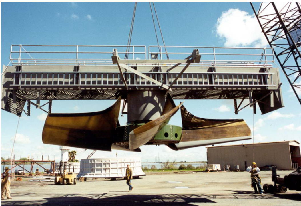
Figure 5. Ultralow Noise Alpina Fan. Photo courtesy of Marley Cooling Technologies.
