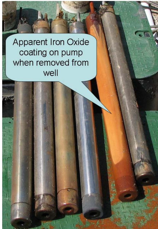
Figure 20. Pumps after approximately 18 months of continuous operation.
