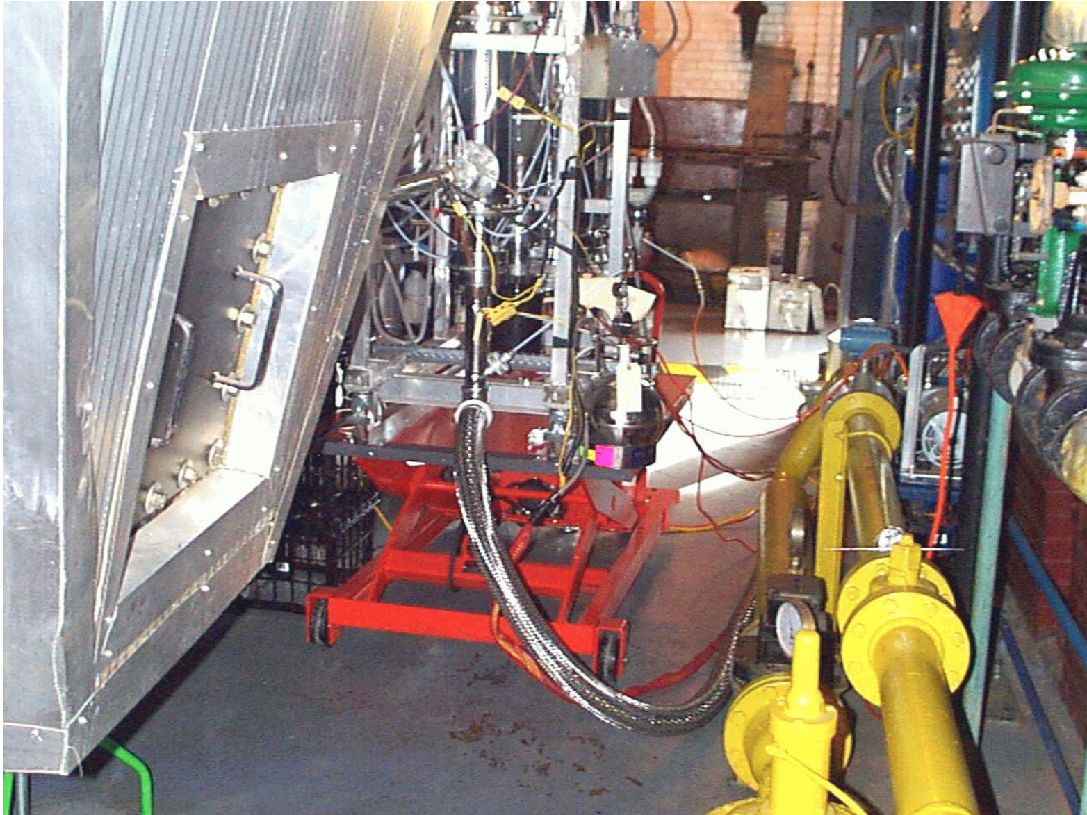
Figure 4-1. Dilution sampling system elevated on mobile lift for access to the sampling port.
