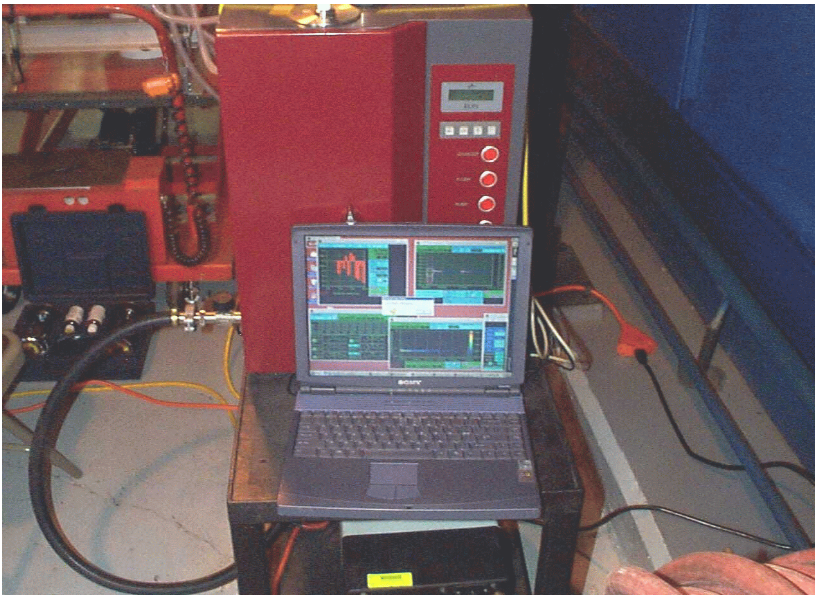
Figure 4-5. ELPI particle sizer positioned at the sampling location (July 7, 2002) for Campaign #2.
