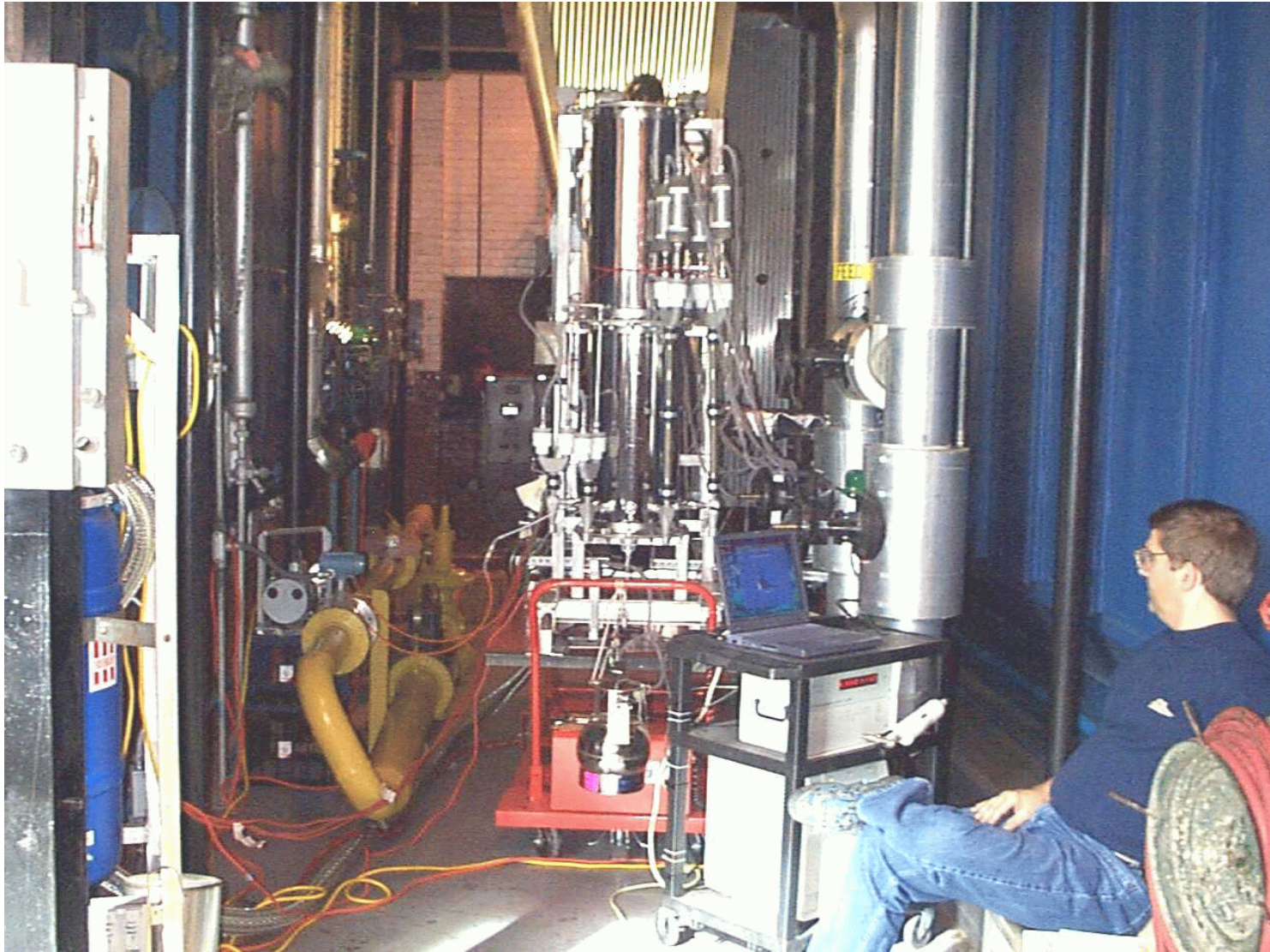
Figure 4-6. Dilution system with all sample collection arrays and instruments attached for Campaign #1.
