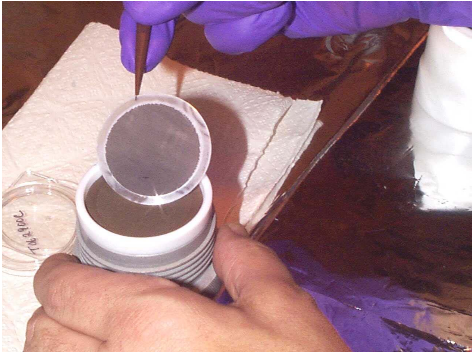
Figure 4-10. Teflon filter being removed from the holder in preparation for packaging for transport to the laboratory.
