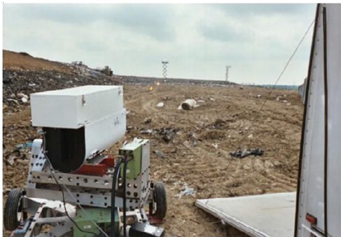
Figure 9. VRPM Configuration Used for the Survey of the Upper Cell During the May 2003 Field Campaign.
