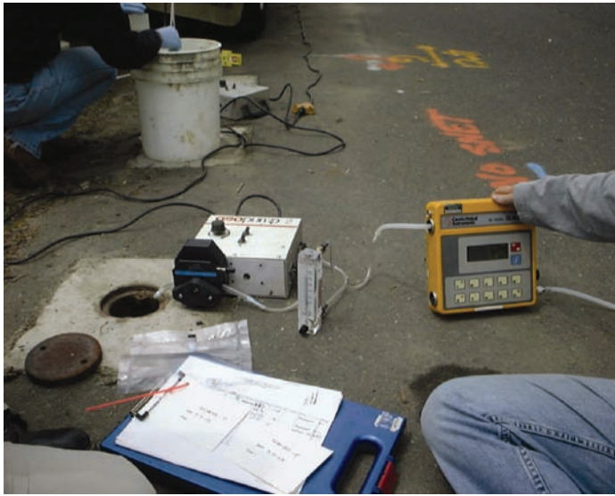
Figure 9. Photograph of peristaltic pump, flowmeter, and landfill gas meter used during purging dedicated vapor probes.
