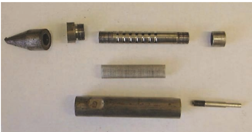
Figure 19. Disassembled view of Retract-A-Tip.
