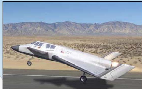
A Concept H2 vehicle is one of three horizontally launched vehicles that will be analyzed in the EIS. Concept H2 vehicles use rocket powered take off and flight and unpowered horizontal landing.
