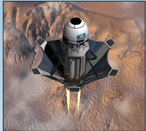
A vertically launched Concept V3 vehicle will be analyzed in the EIS. Concept V3 vehicles consist of a single stage rocket with rocket powered vertical landing. The EIS will analyze a total of six vehicles, three horizontally launched concept vehicles and three vertically launched concept vehicles.
