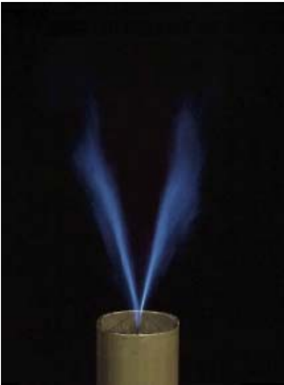
Figure 5. Photograph of an experimental turbulent premixed rod-stabilized “V” methane flame.
