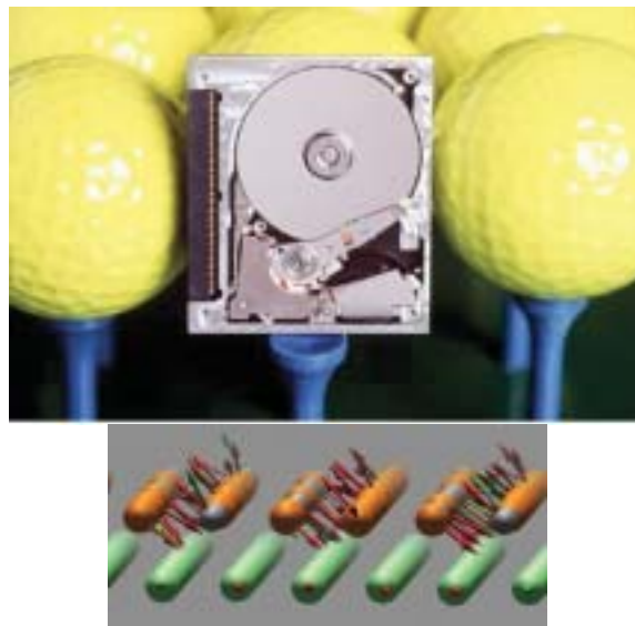
Figure 9. To continue annual doubling of hard drive storage density (top: IBM micro-drive), improved understanding of existing materials and development of new ones are needed. First principles spin dynamics and the use of massively parallel computing resources are enabling researchers at Oak Ridge National Laboratory to understand magnetism at ferromagnetic-antiferromagnetic interfaces (bottom: magnetic moments at a Co/FeMn interface) with the goal of learning how to store binary data in ever smaller domains, resulting in further miniaturization breakthroughs. [M. Stocks]
