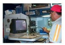
Pollution Control Services (PCS), of Kalkaska, MI, examined the Six-Tile spring water collection complex on July 15 and 16. PCS used a video camera mounted within a waterproof case with interchangeable wheels (for different pipe diameters) to look for breaks that would lead to flow reduction. The camera was connected to a control station via a power/video cable. A remodeled ambulance housed their equipment. Considering the age
